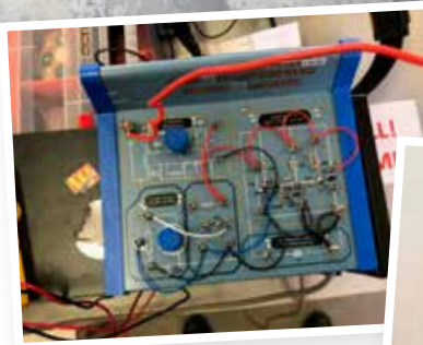
FM radio with external aerial (thicker, red wire)
